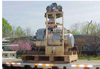
This large bore 24-inch metal seated ball valve was one of several chosen for a tar sands upgrade project. Ability to meet the stringent deadline was crucial to the success of the start-up.
