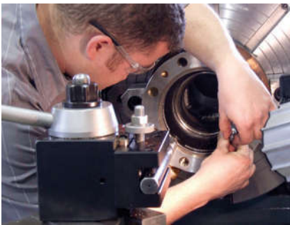
As part of a repair, the MOGAS service technician checks the depth of the seat pocket to certify original design specifications are accurate.
